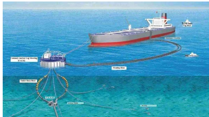
Figure 8: Single Point Mooring (SPM) with Double Pipeline
