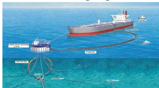
Figure 15: Single Point Mooring (SPM) with Double Pipeline
